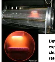
Inside-Gap Plasma Generator for wall cleaning applications
