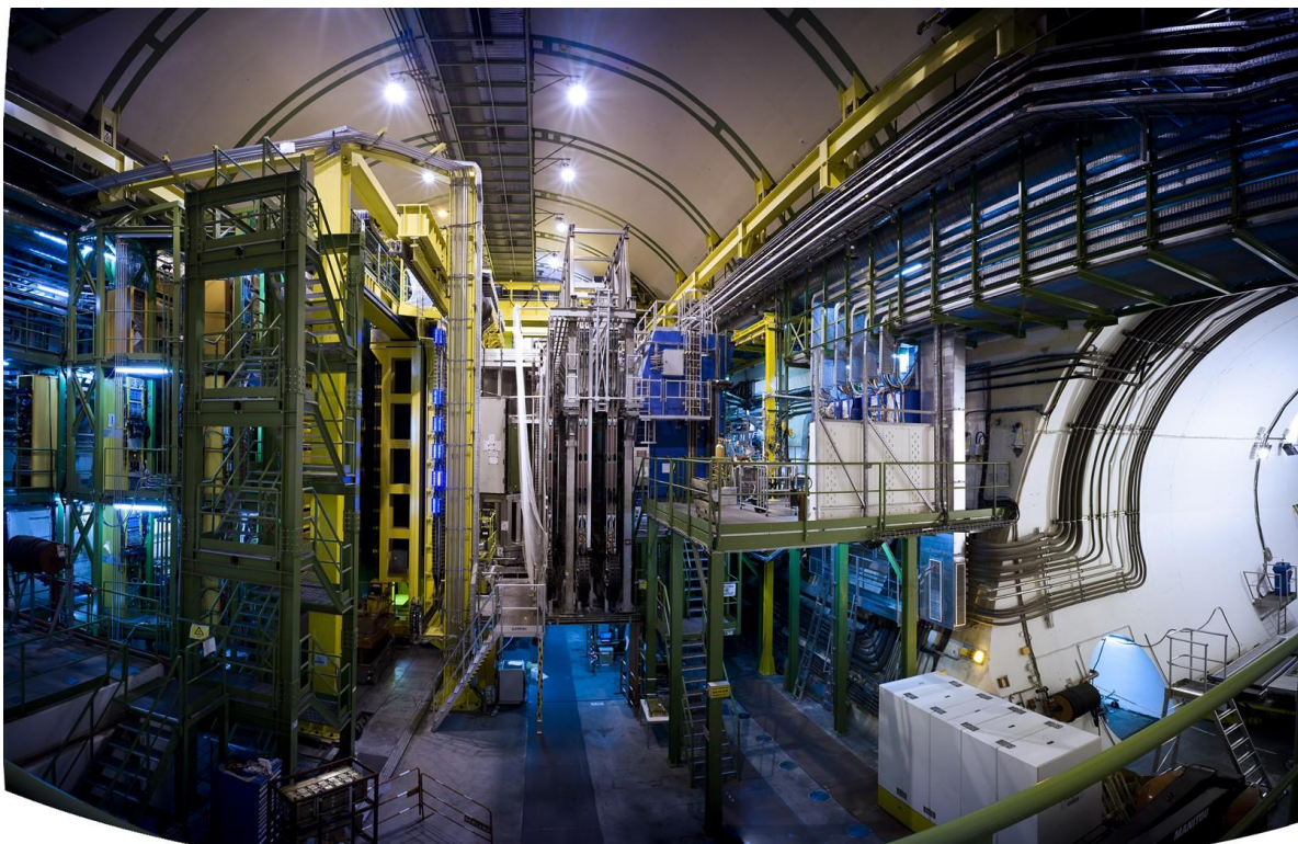
Fig.5 Detectorul LHCb instalat in caverna
