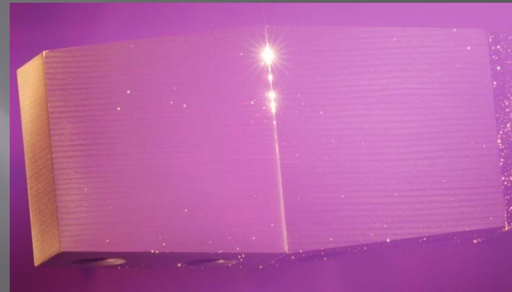
W coated tiles during the HHF test
