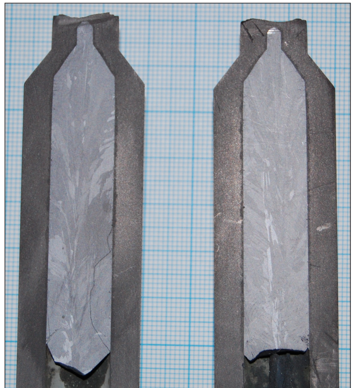
Fig.2. Multicrystalline silicon ingots obtained by Bridgman method
