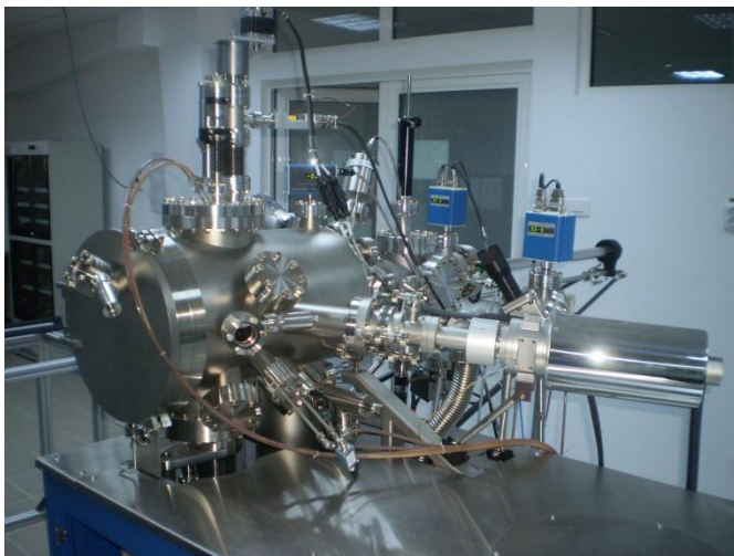
“MBE” Pulse Laser Deposition - Facility for special ultra-thin and thin films depositions -
