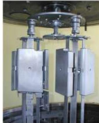
**Tungsten coating of CFC tiles for the JET first wall**
