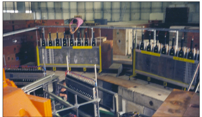
Figure 2. Mounting Preshower Detector at CERN – East Hall
