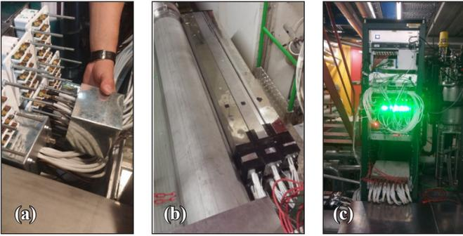
**Fig. 3:** HASC in ECN3 (a) – mounting of fireproof enclosures, (b) – ready for physics (c) – electronics rack
