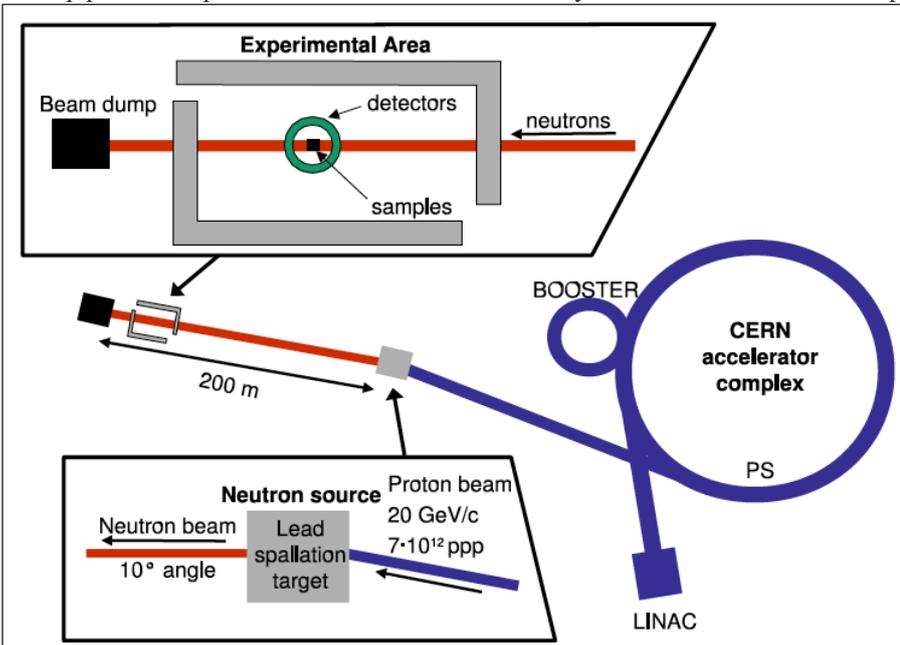
*Fig 1. Left: Layout of the n\_TOF facility within the CERN accelerator complex. Right: Schematic of the two different beam lines of the n\_TOF facility.*
