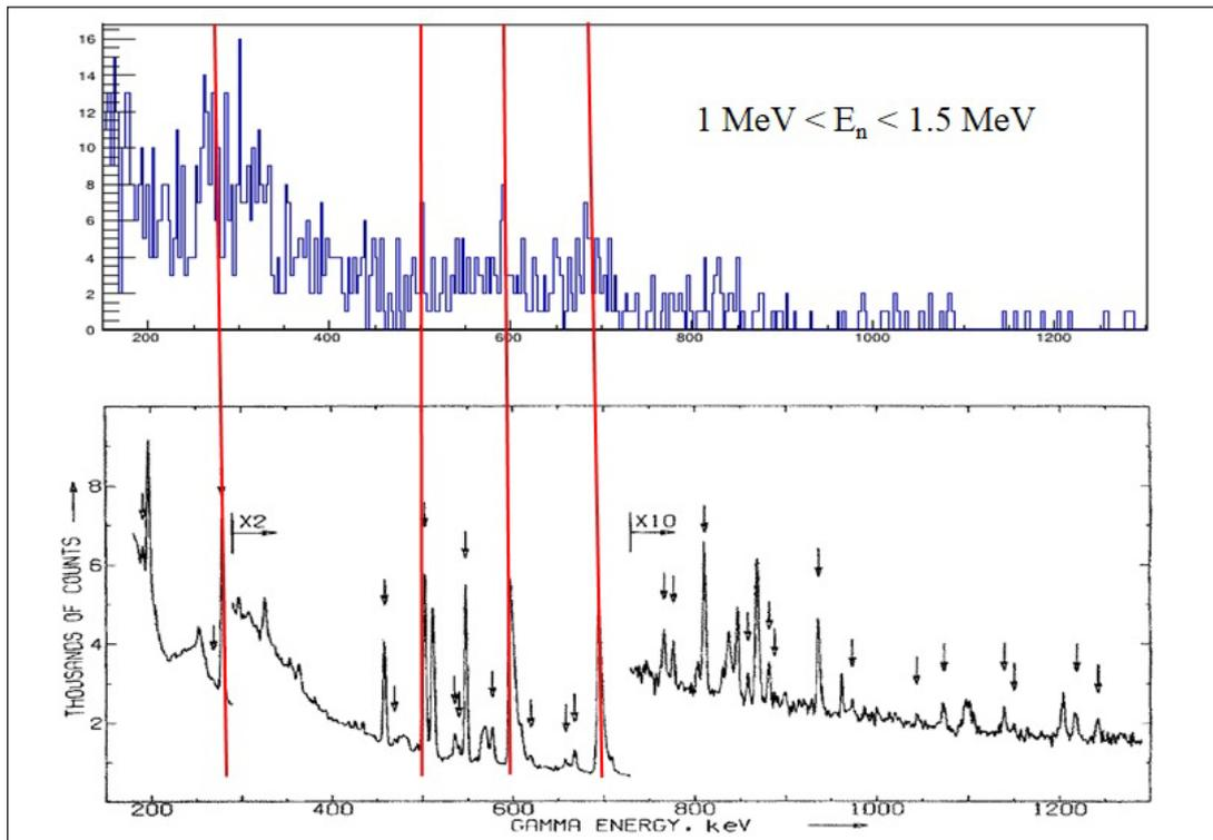
Fig 3. HPGe spectra of a  $^{197}\text{Au}$  sample obtained with the HPGe detector at n\_TOF.
