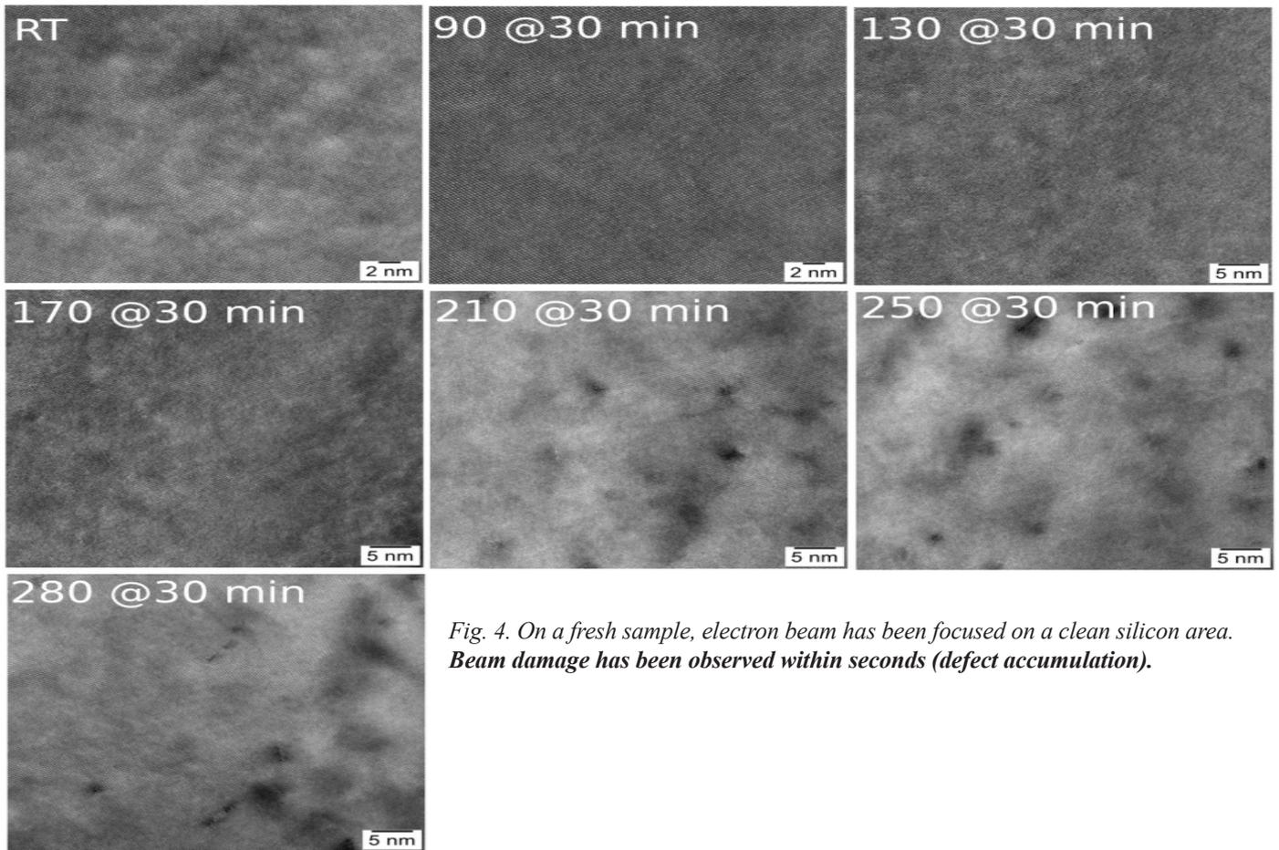
*Fig. 4. On a fresh sample, electron beam has been focused on a clean silicon area. Beam damage has been observed within seconds (defect accumulation).*
