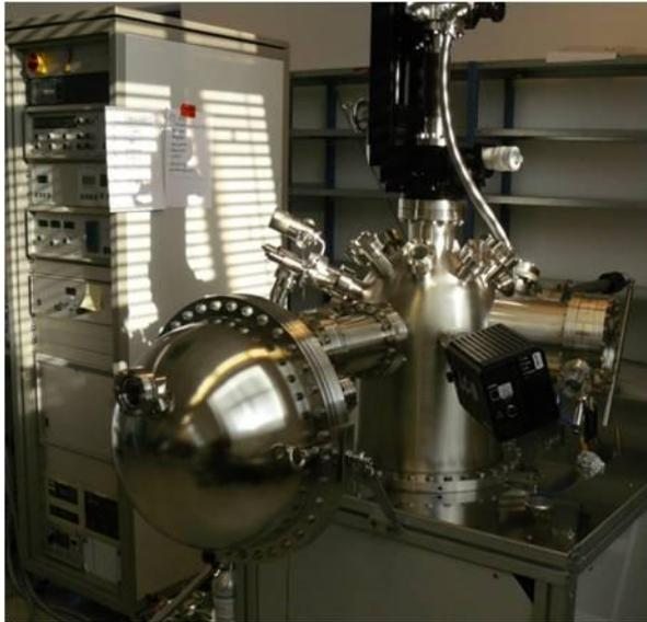
UHV ( $< 2 \times 10^{-10}$  mbar) chamber, a liquid helium-cooled five-axis manipulator and a hemispherical analyser equipped with 2-dimensional detector for energy- and angle-resolved photoemission experiments
