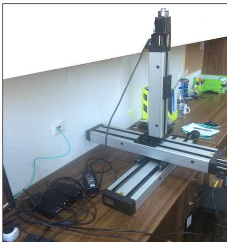
Fig.4. The 3D movement system for the magnetic field measurement.
