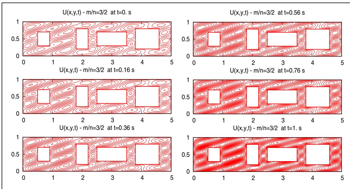
Figure 3. The eddy current stream function  $U(x, y, t)$  at different time, excited by an  $m/n = 3/2$  external kink mode in a thin wall with arbitrary holes.
