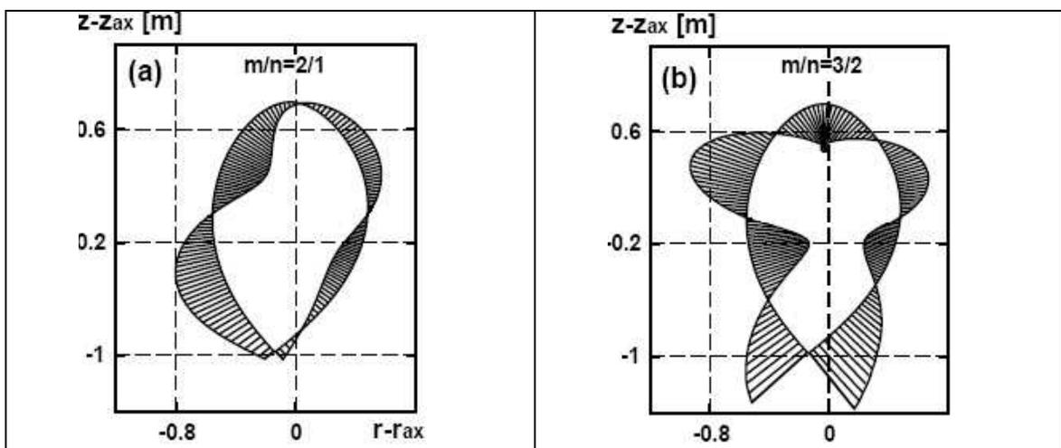
Figure 1. The surface charge distribution along the plasma boundary for unit flux perturbations  $Y_{2/1}$  and  $Y_{3/2}$ , respectively. The plasma configuration of the ASDEX Upgrade tokamak corresponding to the shot no. 13476 at 5.2 s has been considered.
