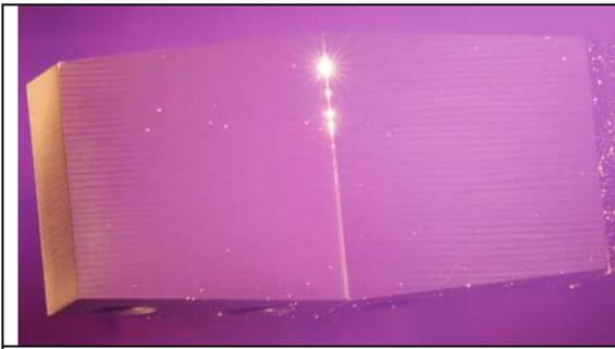
*Figure 3. W coated tiles during the HHF test*
