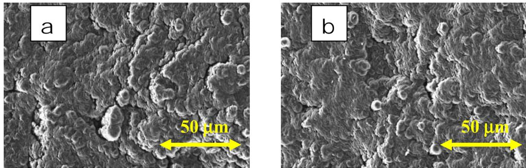
Figure 12. Beryllium coatings on inconel: (a) “as produced”; (b) after HHF test of  $20 \text{ MJ m}^{-2}$ .
