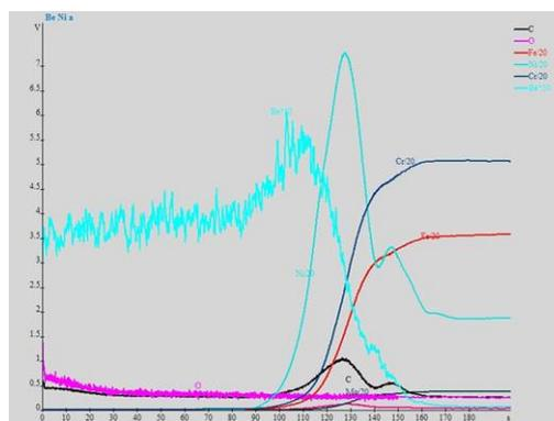
Figure 9. Ni-Be film compositional profile, coated on stainless steel substrate.
