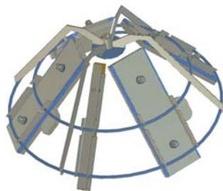
*Figure 1. The design of the new cupola for supporting inconel tiles*
