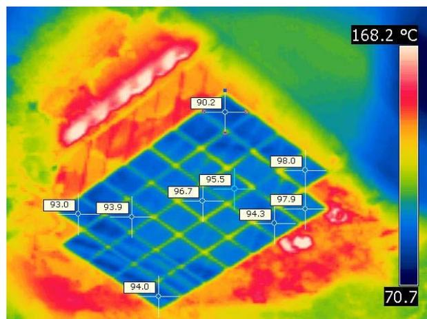
Figure 8. Temperature distribution on the test sample surface ( $94 \pm 4^\circ\text{C}$  thermovision device values, conforming with the real values of  $300^\circ\text{C} \pm 20^\circ\text{C}$ )
