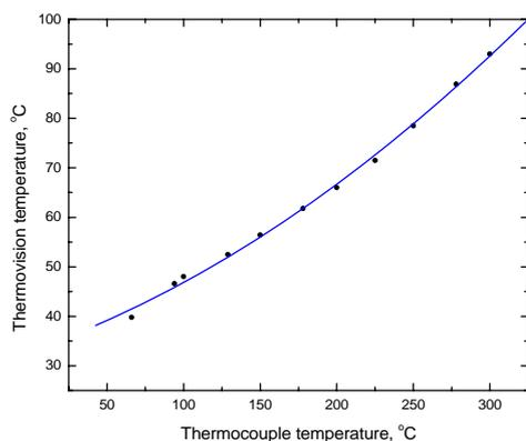
Figure 7. The calibration curve of the thermovision device.
