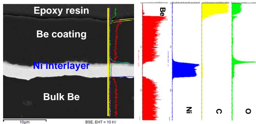
Figure 11. Metallographic cross-section of a marker sample after cyclic test (50 pulses) at  $3.5 \text{ MW m}^{-2}$ .
