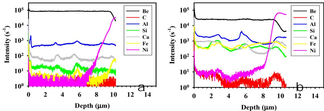
Figure 10. SIMS depth profiles for two markers: a) "as produced"; b) HHF tested at  $40 \text{ MJ m}^{-2}$ .
