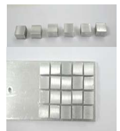
Figure 8. The assembling of castellated surfaces from parts
