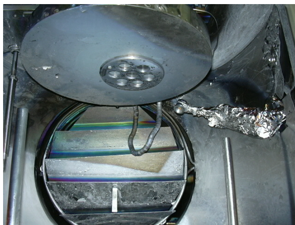
Figure 4. Set-up of the W discs substrate holder and the heating element.
