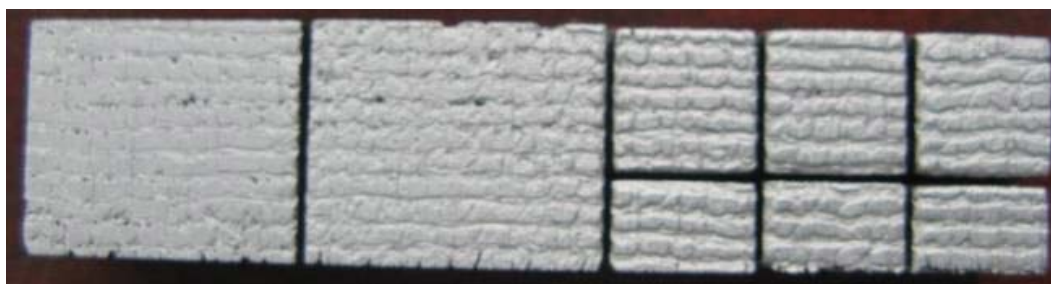
Fig. 6. Be film (100 \mu\text{m} ) deposited on CFC TARCAR target plate parts
