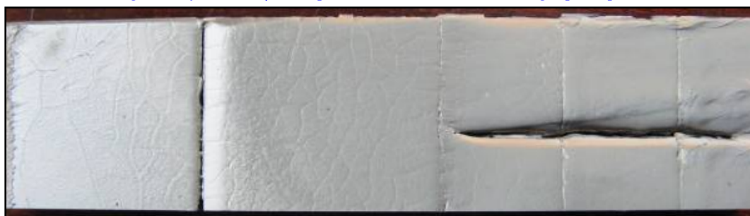
Fig. 6. Be film (100 \mu\text{m} ) deposited on CFC TARCAR target plate parts
