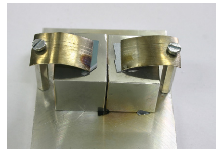
Figure 2: The assembling a two cubes creates a gap. The internal surfaces of the gap are coated with the layer to be removed
