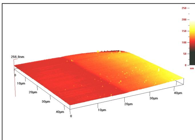
Fig. 7. AFM image of a 100 nm Be/W film coated with 50 nm W coated on Si substrate.
