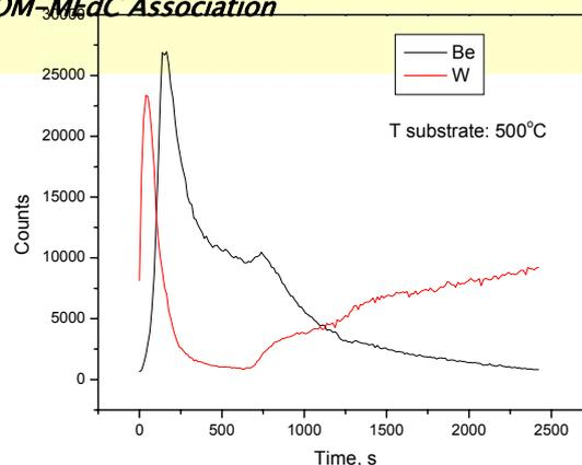
Fig. 10 SIMS depth profile of the Be/W sample deposited at 500°C
