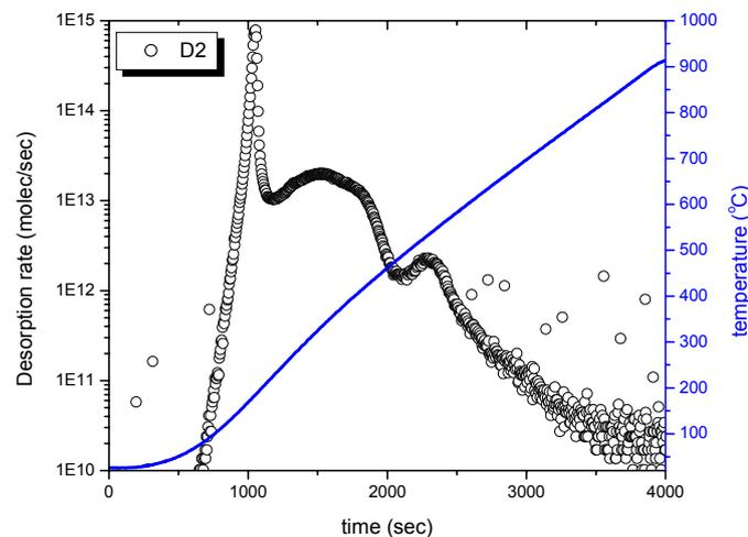
Fig. 12. TDS spectra of a Be-W mixed film deposited on graphite
