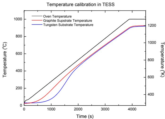
*Fig. 14 Substrate temperature calibration in TESS facility*
