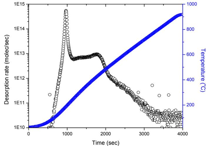
Fig. 11. TDS spectra of a pure Be film deposited on graphite
