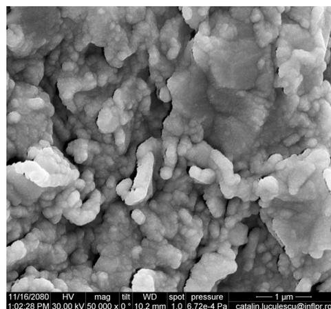
Fig. 3. SEM image of a 300 nm W film coated on C(graphite) substrate
