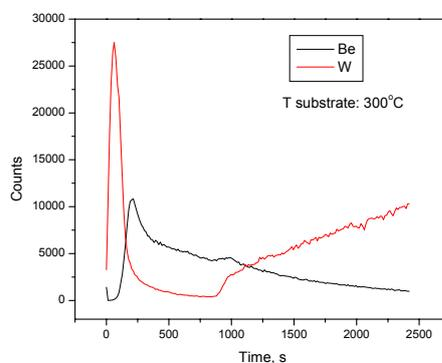
*Fig. 9 SIMS depth profile of the Be/W sample deposited at 300°C*
