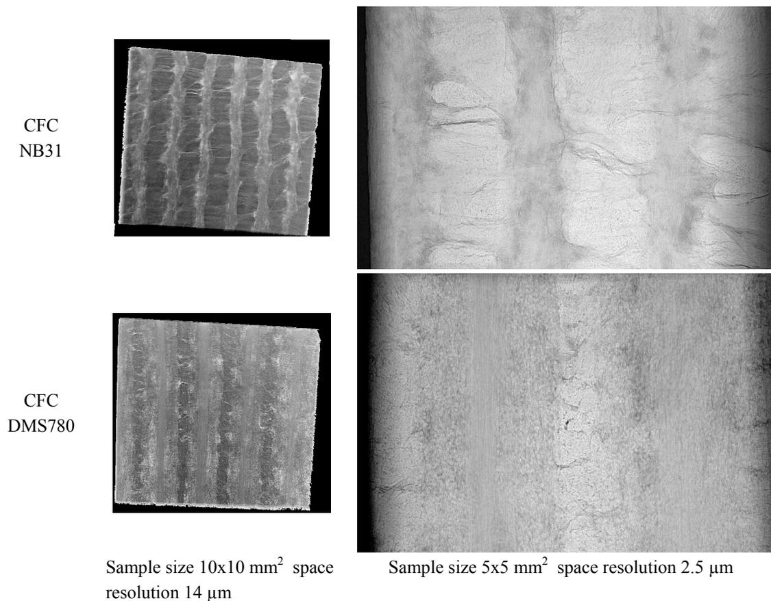
Figure 2: Comparative digital radiographies with space resolution of 14  $\mu\text{m}$  and 2.5  $\mu\text{m}$
