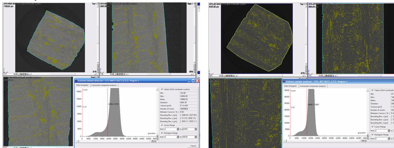
CFC NB31: 6 μm/voxel; porosity factor 8.05%
