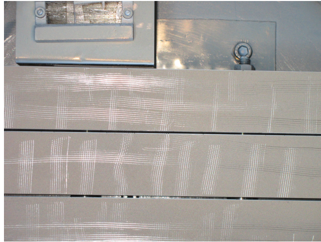
Fig.5 Scratching traces of the Be test tiles after the adherence test.
