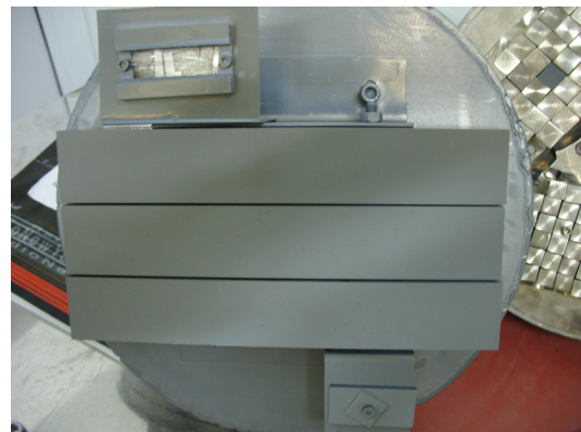
Fig.4 Be tiles after Ni+Be deposition
