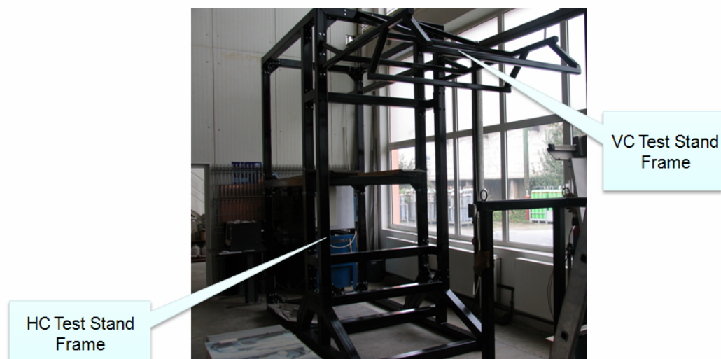
Figure 6 the manufactured KN3-NA Test Stand
