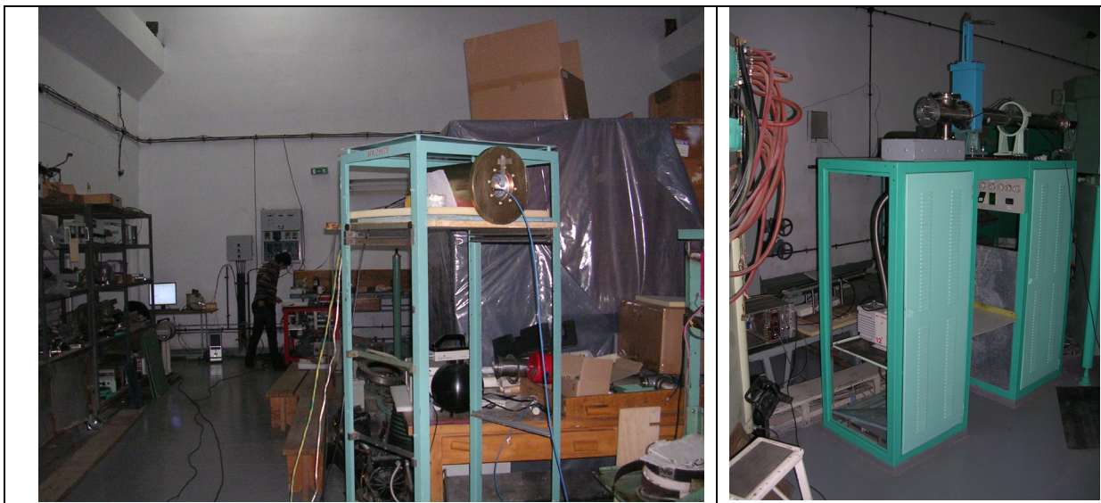
Fig. 1. LaBr 3 detector (left), situated at a distance of 3 meters from the aluminum target (right).
