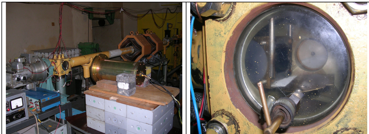
Fig. 10. \text{LaBr}_3 detector at the cyclotron accelerator (left) and the beryllium foil, seen as a darker surface, inside the irradiation chamber (right).
