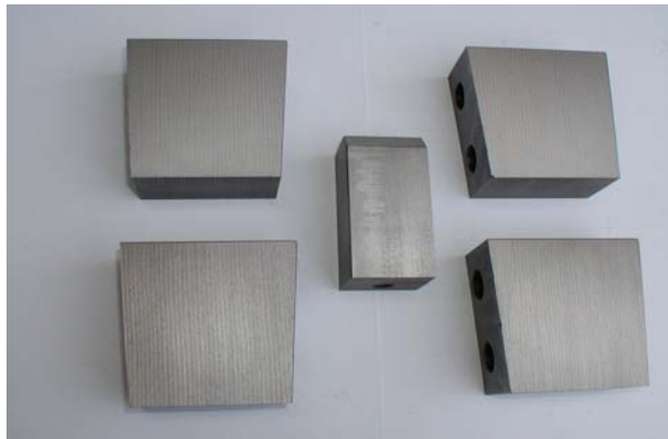
Figure 10. The CFC tiles coated by CMSII technology with 10 \mu\text{m} tungsten, which have been sent to IPP Garching for testing
