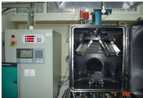
Thermal evaporation system dedicated for Inconel tiles coating. Below: Inconel IGWL and IWC tiles coated with Be by thermal evaporation, Inconel DPC tiles coated with Be by thermal evaporation
