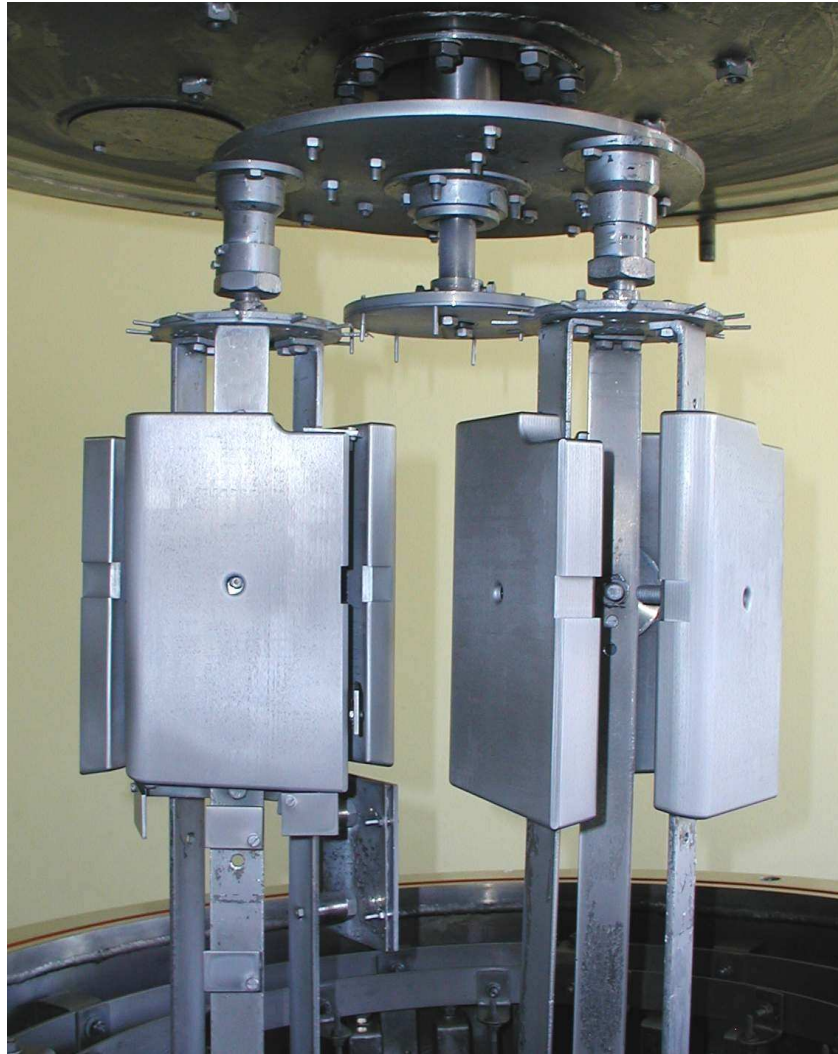
Fig.3 Inner Wall Cladding W coated prototypes tiles for JET
