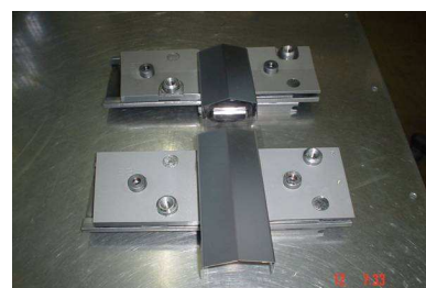
Thermal evaporation system dedicated for Inconel tiles coating. Below: Inconel IGWL and IWC tiles coated with Be by thermal evaporation, Inconel DPC tiles coated with Be by thermal evaporation
