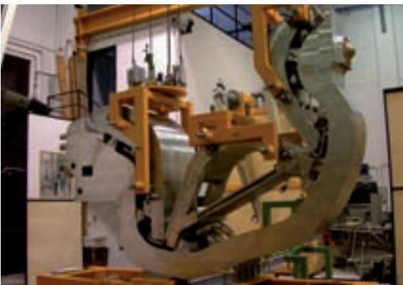
Image 2 Integrated Divertor Cassette (Courtesy ENEA)
