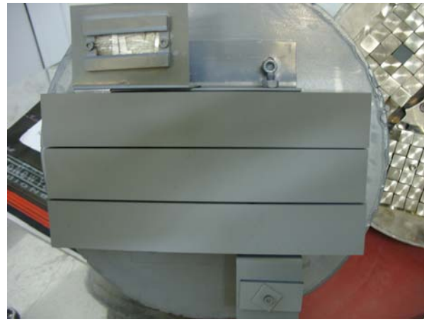
Fig.4 Be tiles AFTER Ni+Be deposition
