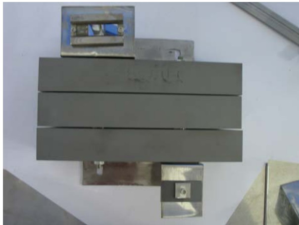
Fig.3 Be tiles BEFORE Ni+Be deposition
