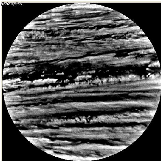
Figure 9 – Tomographic analysis of the tungsten coated CFC region of ITER-like wall sample: 2D image of the tungsten layer (top-left) and two orthogonal views of the tungsten layer (second and third rows). Bright regions correspond to tungsten. The total thickness of the tungsten layer and the Mo buffer are evaluated at around 12 microns (bottom image).
