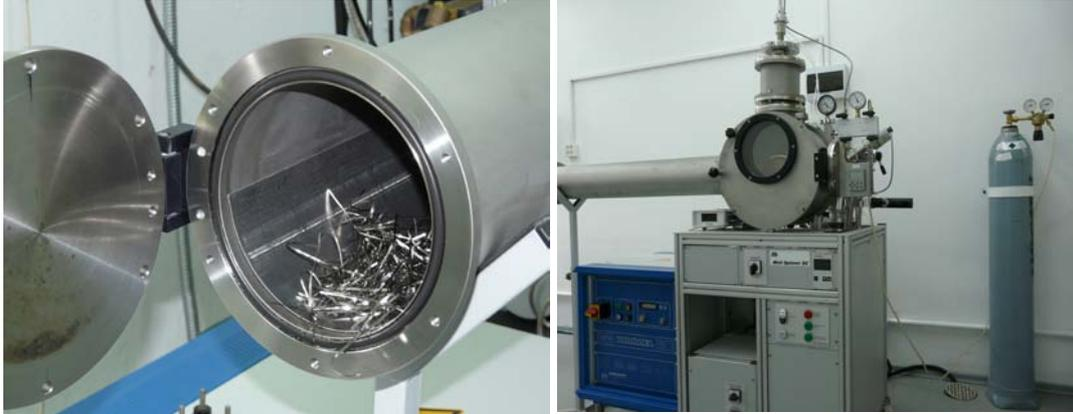
Figure 2. Melt spinning apparatus used for sample preparation.
