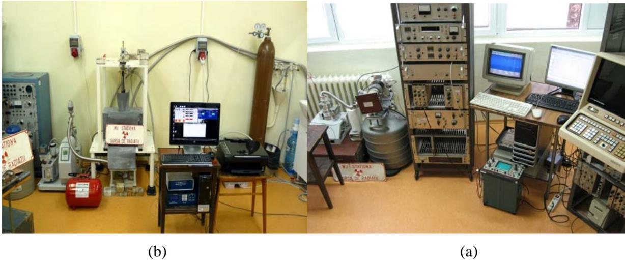
Figure 2. Laboratory Mössbauer spectrometers: a) Promeda spectrometer; b) See Co spectrometer.
