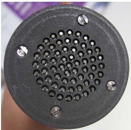
Fig. 1. Front picture of the multi-probe system with 61 collectors
