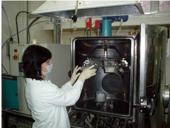
Fig. 5 Adjusting Inconel tiles on the jigging device
