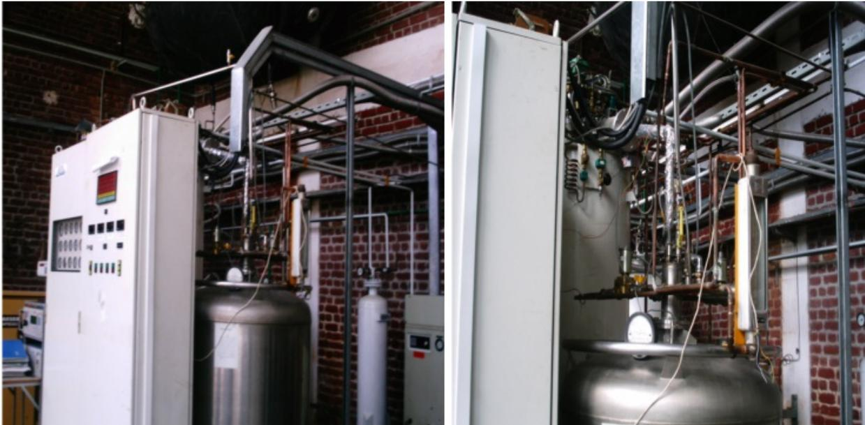
Figure 1: Linde L5 Helium liquefaction system in Low-temperature Lab of ICIT Ramnicu Valcea
