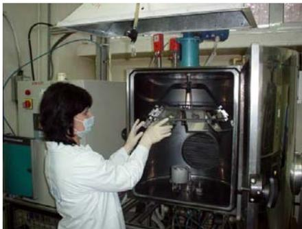
Figure 5 – Adjusting Inconel tiles on the jigging device
