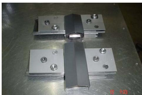
Figure 1 – Inconel IWGL tiles coated with Be by thermal evaporation in vacuum method
