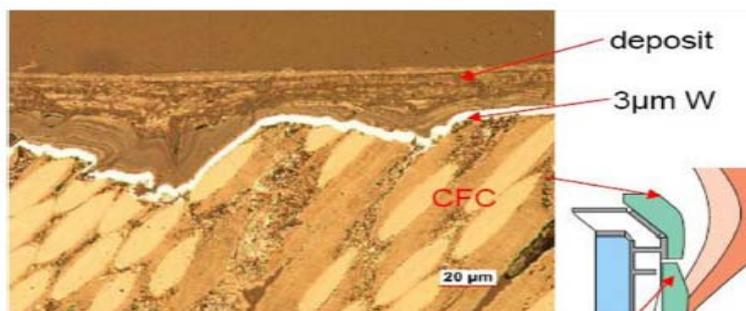
Figure 6 - Cross-sectional profile of the tile 1 from the campaign 2001-2004 [5].
