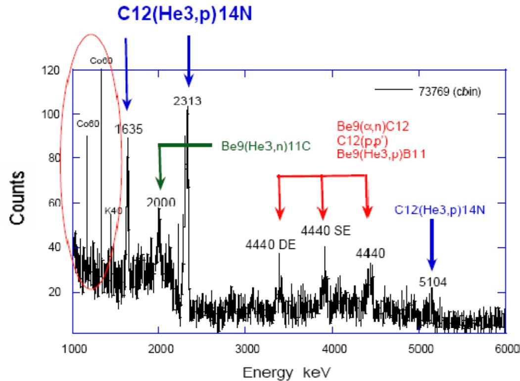
$\gamma$  spectrum of a JET D( $^3\text{He}$ ) discharge with ICRH @  $\omega = \omega_{\text{C}^3\text{He}}$
