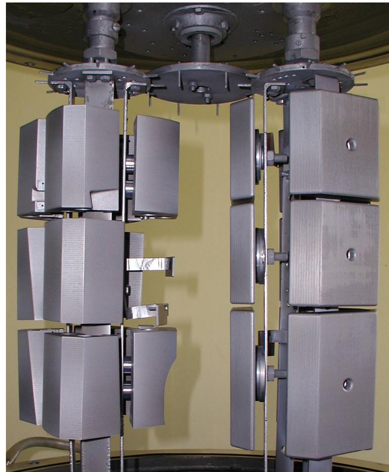
IWGL (Be) from the main chamber; coating thickness 10-15  $\mu\text{m}$
