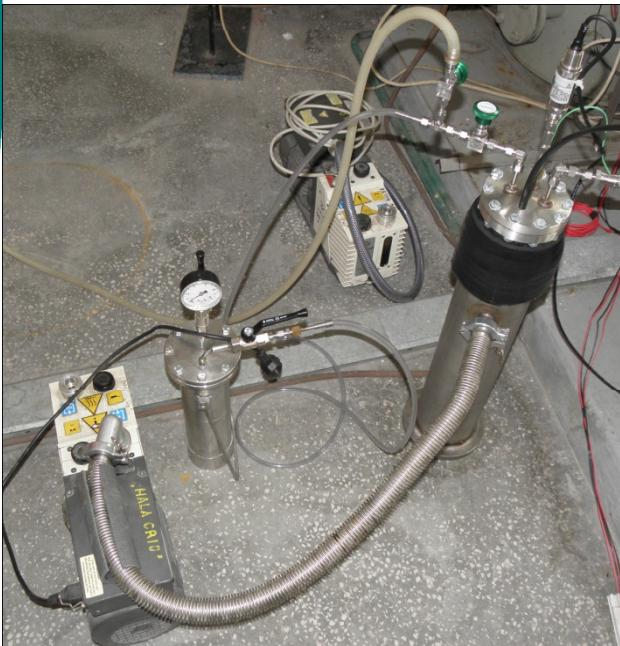
Minimum Absorption Rate Determination Rig
