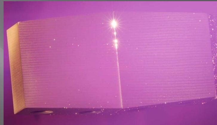
W coated tiles during the HHF test
