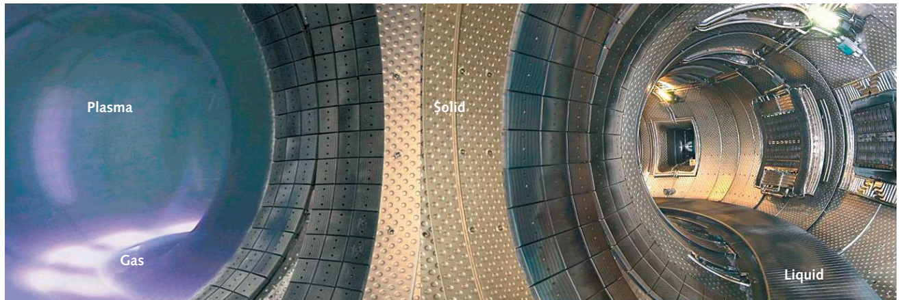
Where the four states of matter meet: Plasma, gas, solid and liquid are all present in a fusion reactor. The left side of this internal view of the Tore Supra tokamak shows a superimposed view of the machine in operation. The bright zones correspond to areas of strong plasma wall interaction. The plasma facing components are cooled by water flowing only a few millimetres below their surfaces. (Photo: CEA)
